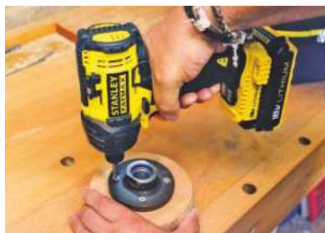
▲ The impact driver was at home with small screws here or 100mm ones directly into beech
